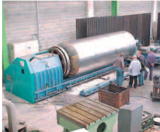
Delivery of the new winding mandrel for the Zefiro 23 motor of the second stage of the Vega small launcher (Courtesy of Avio)
