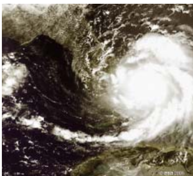
Two views of Hurricane Katrina acquired on 28 August 2005 with instruments onboard Envisat. The ASAR radar image of the sea surface (left) shows how Katrina's wind fields caused rippling of the ocean surface. The MERIS optical image (right) shows characteristic swirling cloud patterns around the central eye, with the eye 'walls' also visible
