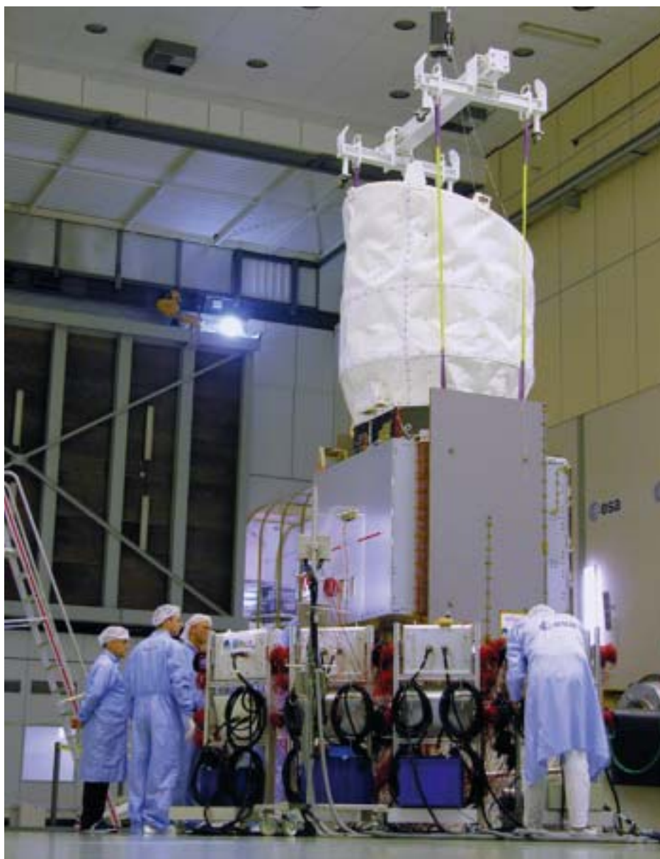
The structural model of ADM/Aeolus mounted on the multi-shaker in the ESTEC Test Centre
