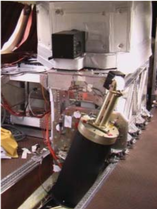
The Aladin Airborne Demonstrator mounted in the DLR aircraft for in-flight testing
