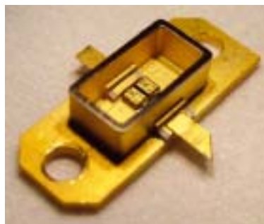
Wide-bandgap technology: a package containing two parallel, 12 x 125 micron, high-gain, high-efficiency microwave transistors
