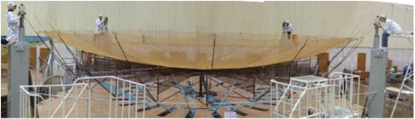
Reflector surface-accuracy measurements in progress on a large deployable antenna (Courtesy of NPO-EGS, RSC Energia and Alcatel Alenia Space Italy)
