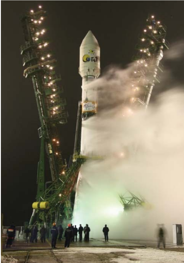
The Soyuz 2-1b + Fregat combination carrying COROT about 15 min before launch as the gantry was being moved away
