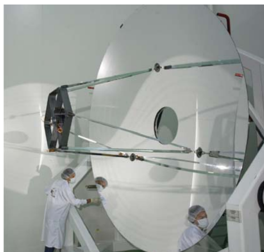
The Planck telescope with videogrammetry targets mounted
