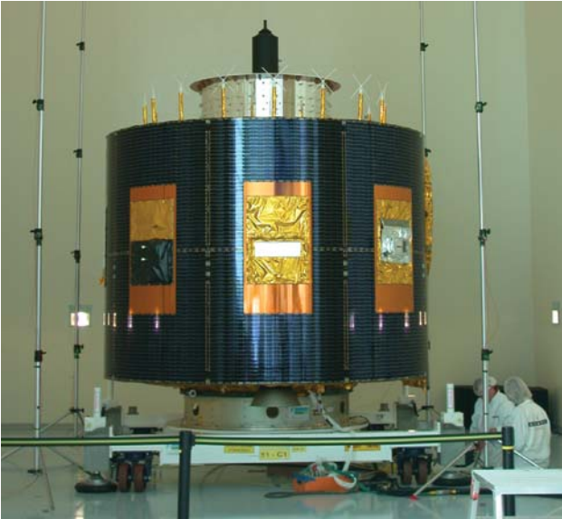
The MSG-4 spacecraft being prepared for acoustic vibration testing at Alcatel Alenia Space in Cannes (F) (Photo: AAS, Cannes)
