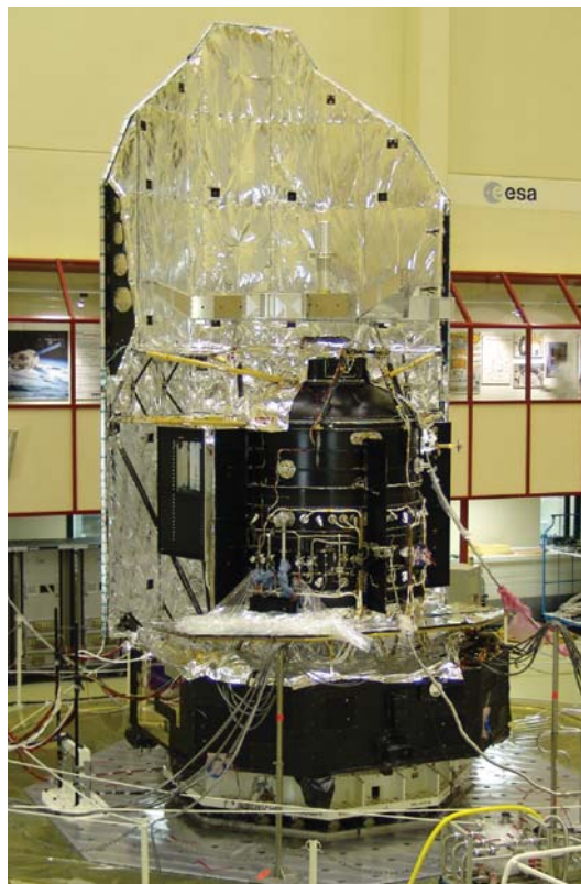
The Herschel structural model on the Hydra test facility at ESTEC (NL)
