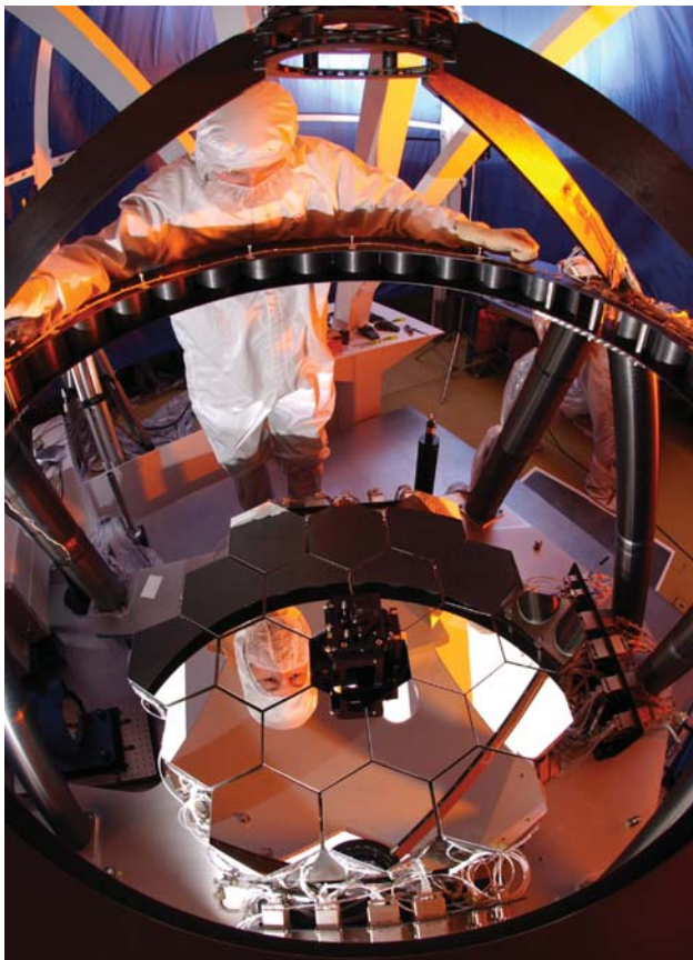
JWST wavefront sensing and control testbed to demonstrate the feasibility of the active alignment approach for the main telescope. The testbed is a scaled-down model of the full telescope, including actuators
