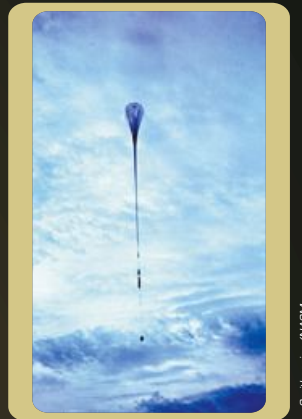
Observations with infrared telescopes carried by balloons started in the sixties. These balloons reached altitudes of more than 40 kilometres and helped to overcome some of the worst problems associated with atmospheric absorption.
