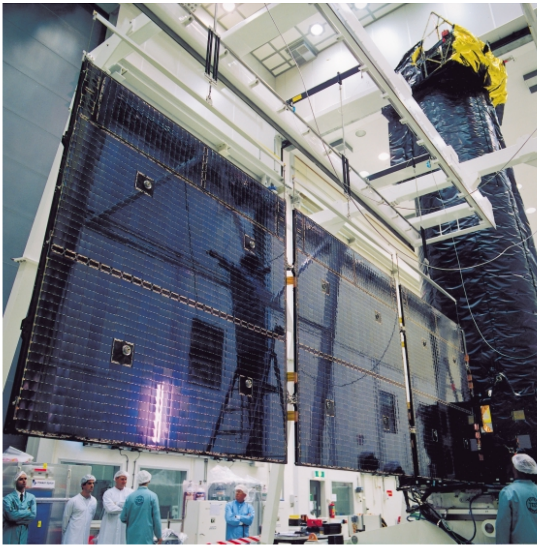
Figure 2. One of XMM's two solar-array wings (flight model), each of which has three folding rigid panels
