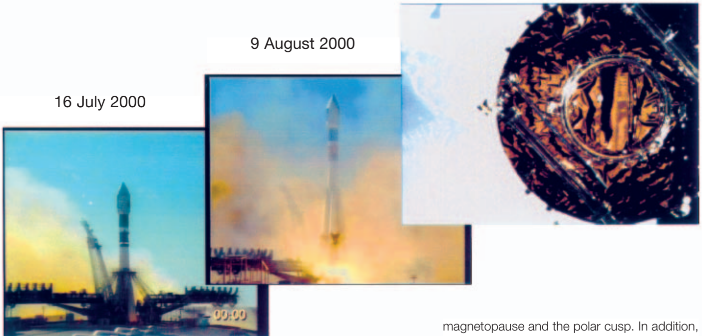
Figure 1. The two launches of the Cluster spacecraft on two Soyuz-Fregat rockets, on 16 July and 9 August 2000. An onboard camera took 27 pictures when Rumba-SC1 separated from Tango-SC4. Tango is shown in the upper-right corner. The Earth can be seen in the background
