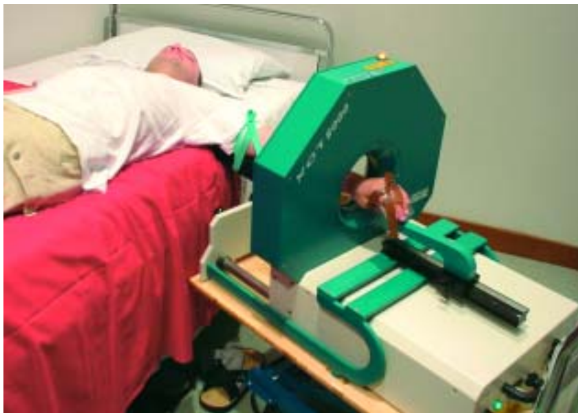
Figure 7. Localised QCT: high resolution analysis and imaging of a slice of the forearm
