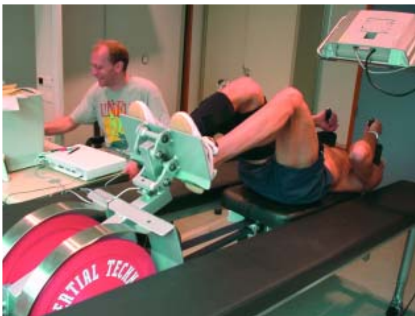
Figure 5. The exercise countermeasure – leg force pushing a set of flywheels
