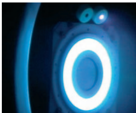
The SMART-1 thruster during firing tests at SNECMA (F)
