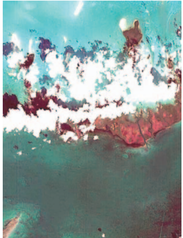
Image of the coast of Cuba reconstructed from data in three spectral bands acquired with PROBA's CHRIS instrument
