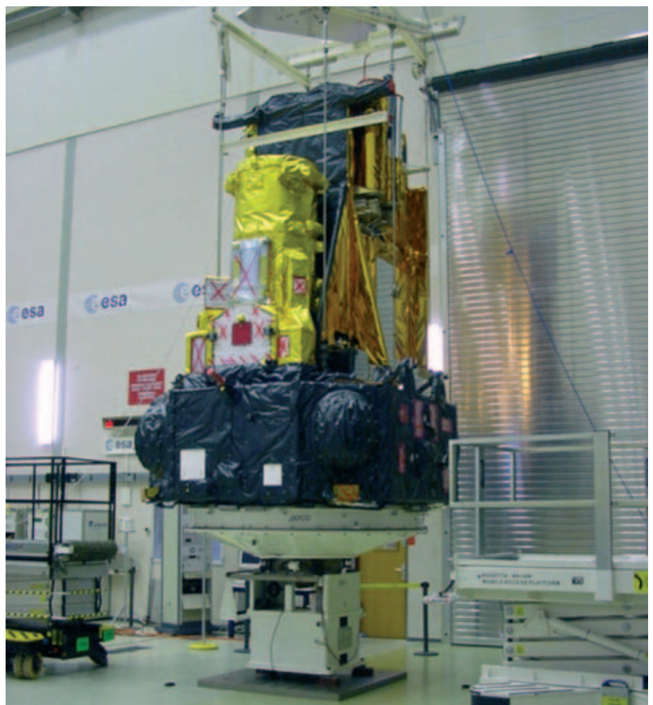
Integral undergoing mass-properties testing at the end of the environmental test campaign at ESTEC in Noordwijk (NL)
