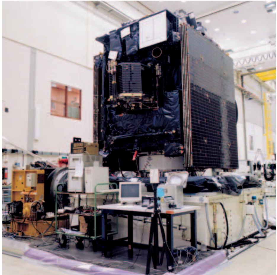
The Rosetta flight spacecraft on the vibration shaker at ESTEC in May 2002
