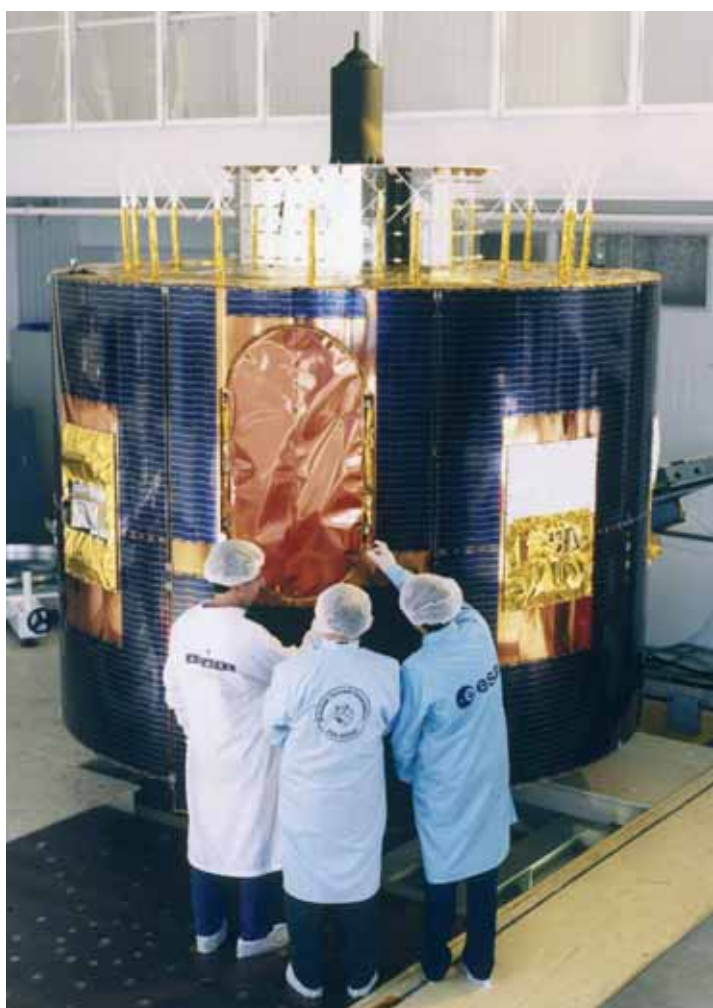
The MSG-1 satellite's final inspection before launch (photo courtesy of Alcatel Space Industry, Cannes)
