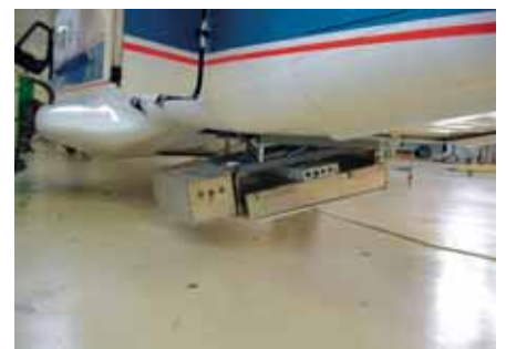
The STARRS instrument mounted beneath DLR's Dornier 228 aircraft for the ESA EuroSTARRS campaign
