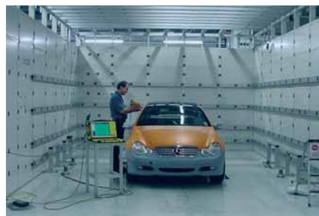
Preparing for ProCam measurements on a vehicle to be crash-tested with reference points on the walls of the measurement chamber
