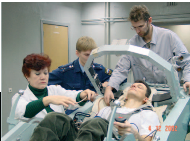
About to go into the centrifuge for an 8-g test
