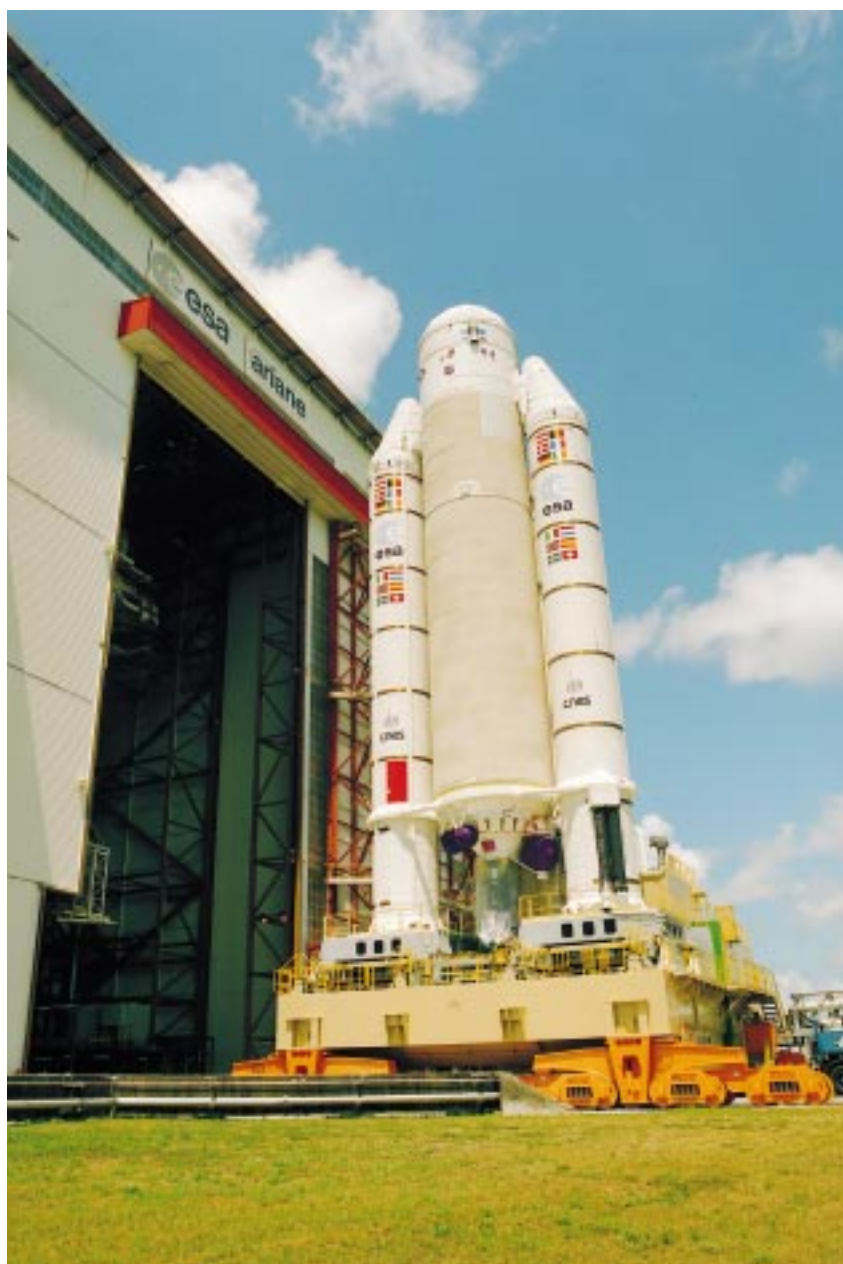
Transfer of the Ariane-503 lower composite from the Launcher Integration Building to the Final Assembly Building on 3 October
