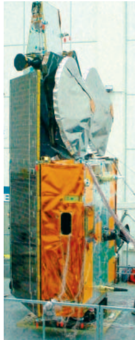
CryoSat on the shaker at ESTEC for vibration testing
