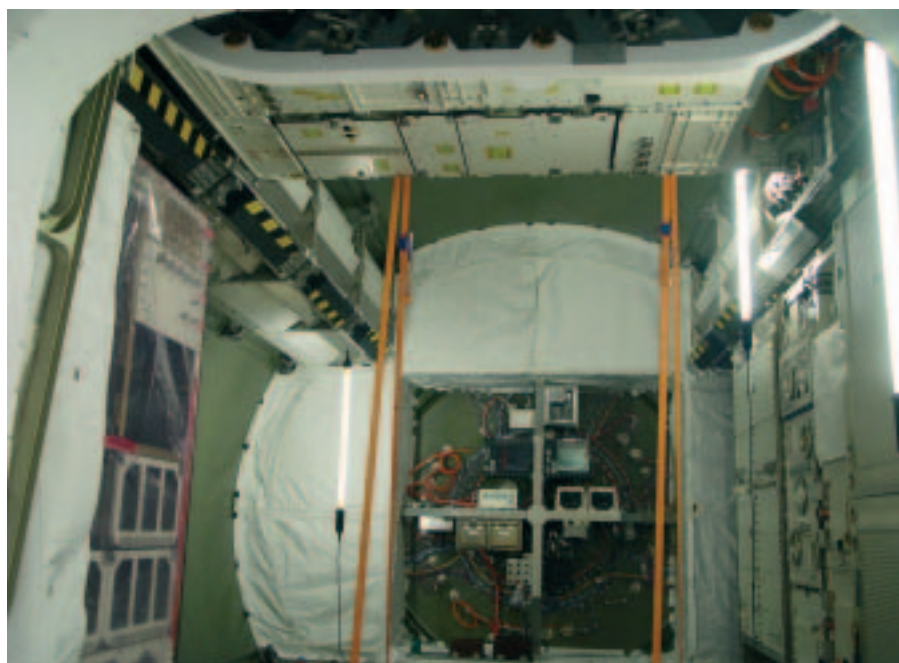
The flight models of the pressurised payloads inside Columbus during IST testing in Bremen
