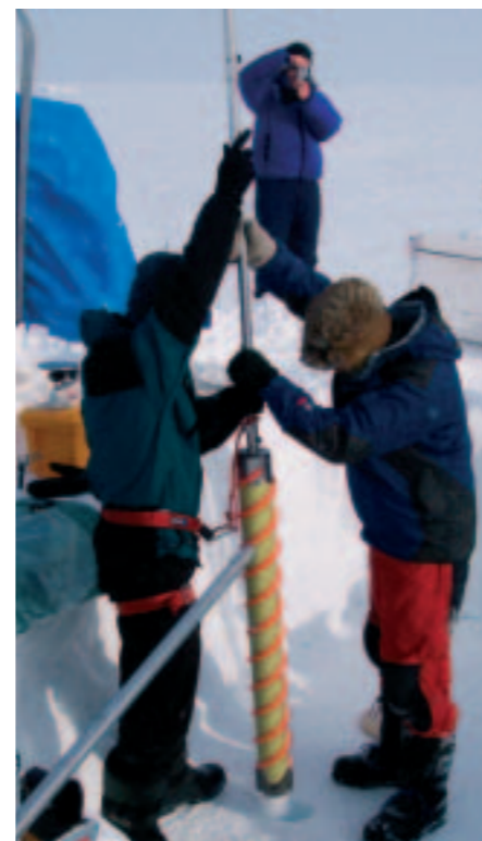
Drilling cores into the ice sheet to measure fluctuations in snow fall and near-surface density
