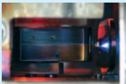
A caesium ion slit emitter during validation testing for LISA
