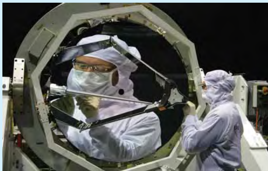
The ALADIN primary mirror during inspection at Astrium Toulouse
