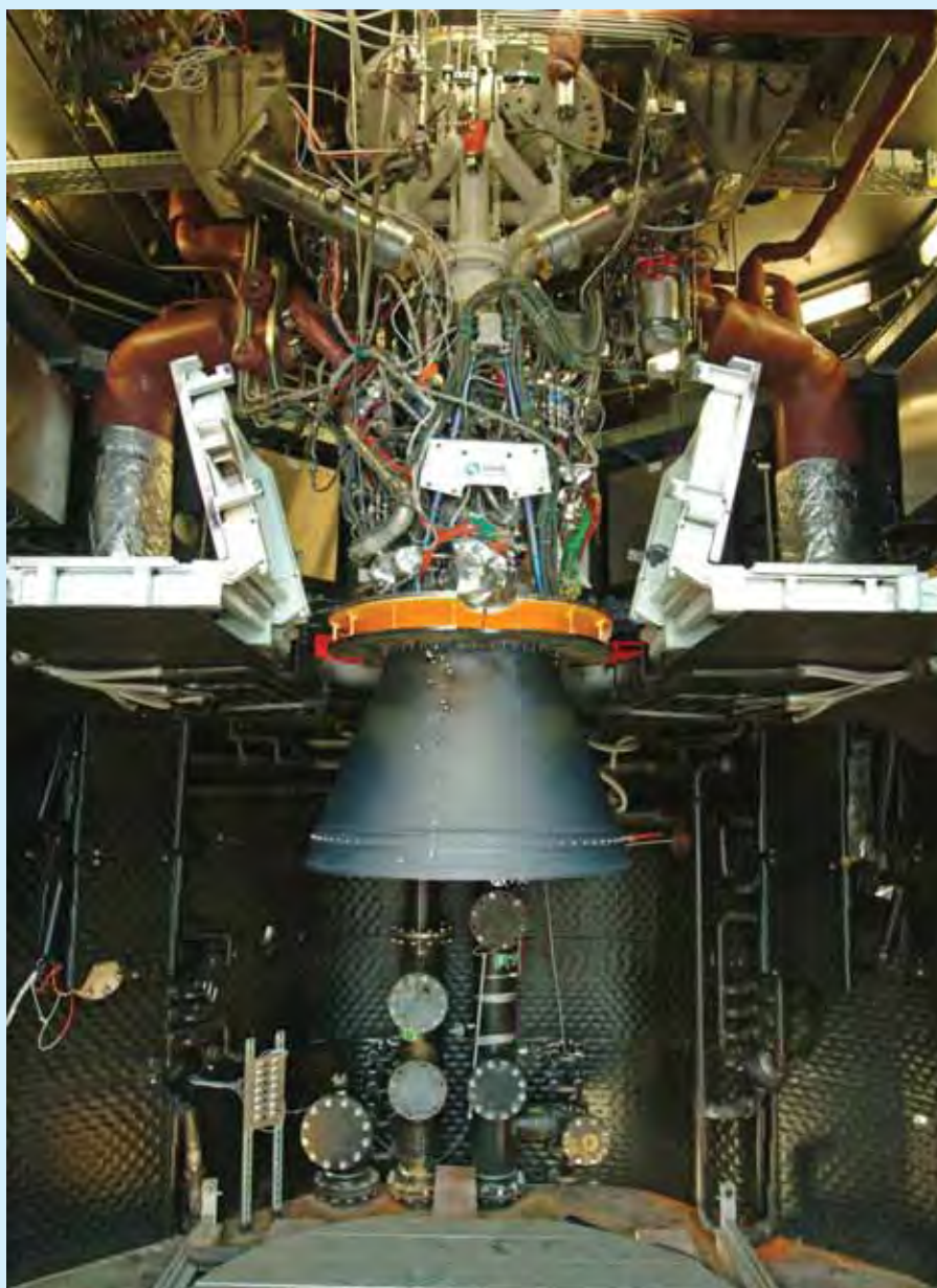
The FLPP Expander Demonstrator engine on teststand P4.1 at Lampoldshausen, Germany
