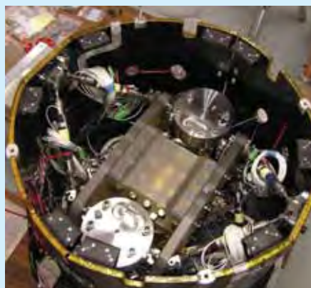
The LISA Technology Package Central Assembly mounted inside the LISA Pathfinder science module flight structure under vibration test at Astrium GmbH in Friedrichshafen
