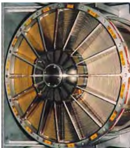
An XMM-Newton mirror module comprising of 58 nested mirror shells (ESA/Dornier Satellitensysteme GmbH)
