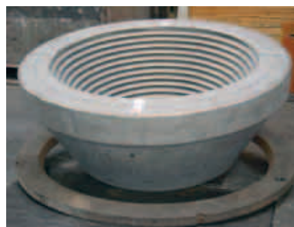
The forging for the dome structure, and after machining.
