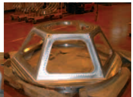
The forging for the dome structure, and after machining.
