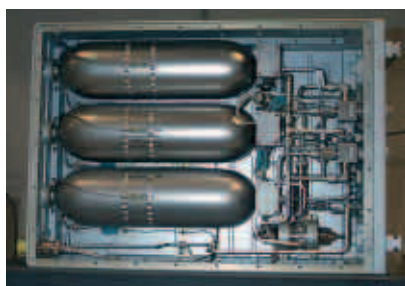
MSL-USLab Gas Supply drawer Flight Model (bottom view, cover plate off).
