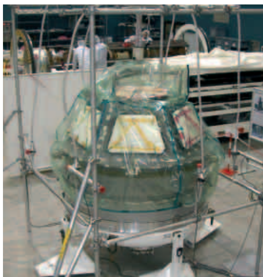
Testing the pressure integrity of the whole Cupola.
