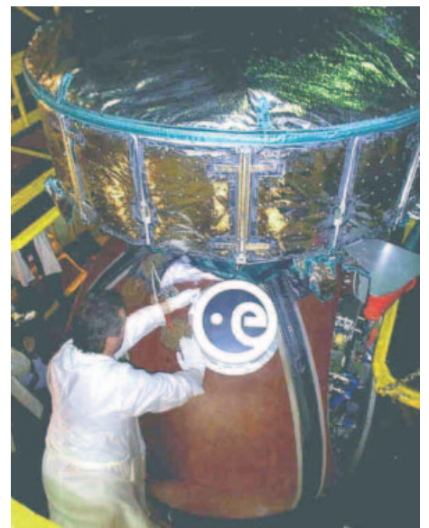
ESA's Moscow Office supported the Foton-12 team in Russia. Biopan is seen here being installed on the return capsule.
