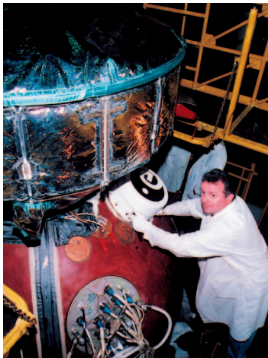
Fig. 2. Biopan integrated on the Foton descent capsule.
