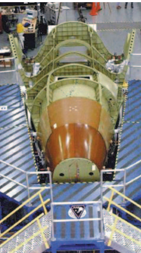
The V201 space-test X-38 prototype is under assembly at NASA's Johnson Space Center.
