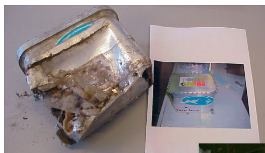
The remains of a Biofilter from Foton-M1.
