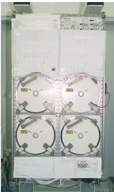
MELFI FU1 at KSC ready for integration in the MPLM. An acoustic blanket is installed on the upper part.
