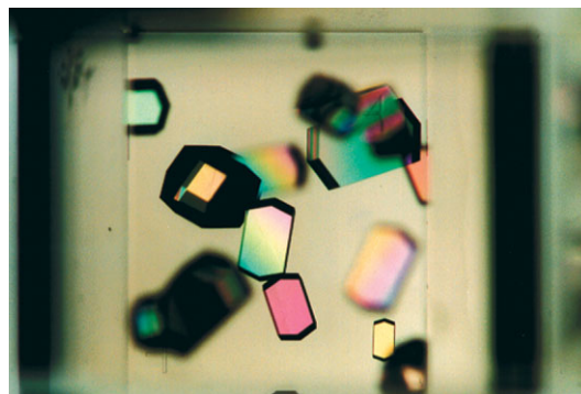
Crystals grown on APCF during the Spacehab/STS-95 mission in October 1998. (ESA)
