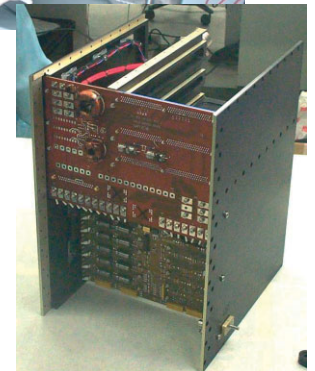
Hexapod Electronic Unit during integration.
