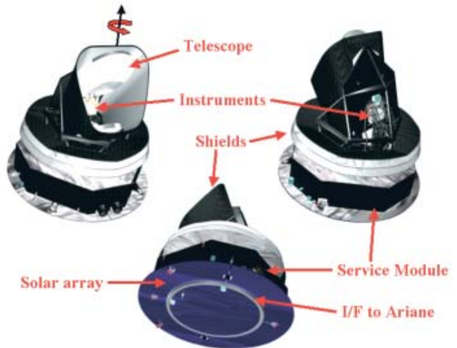
Figure 4.2.1. The current configuration of the Planck satellite, as developed by Alcatel Space (F).
