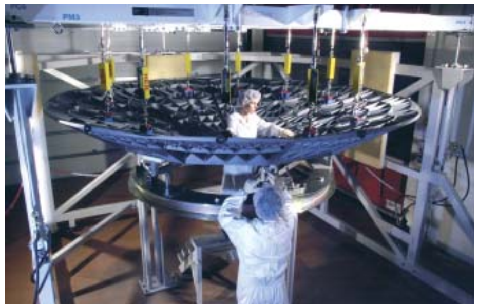
Figure 4.1.2. Herschel's primary mirror blank, shown just after the brazing together of 12 individual SiC segments to form a monolithic structure was completed in late 2003. This mirror blank will now be ground, polished and coated in the course of 2004. (EADS Astrium)
