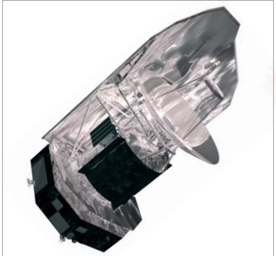
Figure 4.1.1. The Herschel satellite in orbit. Clearly visible are the passively cooled telescope behind its protective sunshade, the superfluid helium cryostat containing the science instruments, and the service module. (Alcatel Space Industries)
