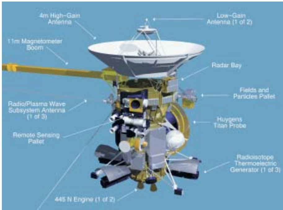
Figure 2.4.4. The Cassini/Huygens spacecraft and its principal features.
