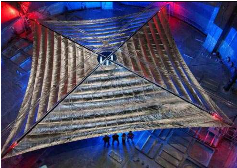
Figure 7.2: 2004, 20×20 m solar sail ground test (NASA/AEC)
