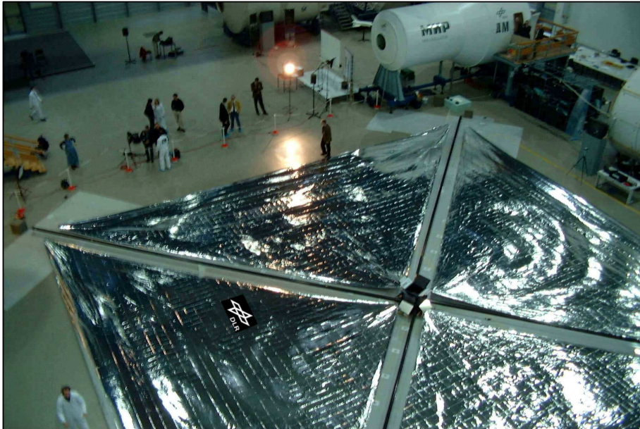
Figure 7.1: 1999, 20×20 m solar sail ground test (DLR/ESA)
