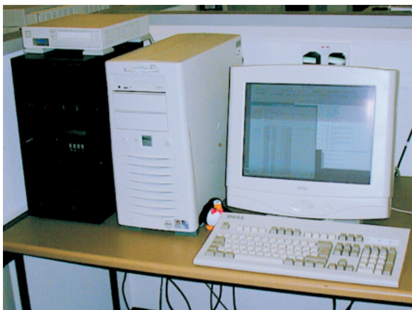
Figure 3. The scheduler subsystem of the UK-PAF. The black unit on the left is the RAID unit, providing full data redundancy
