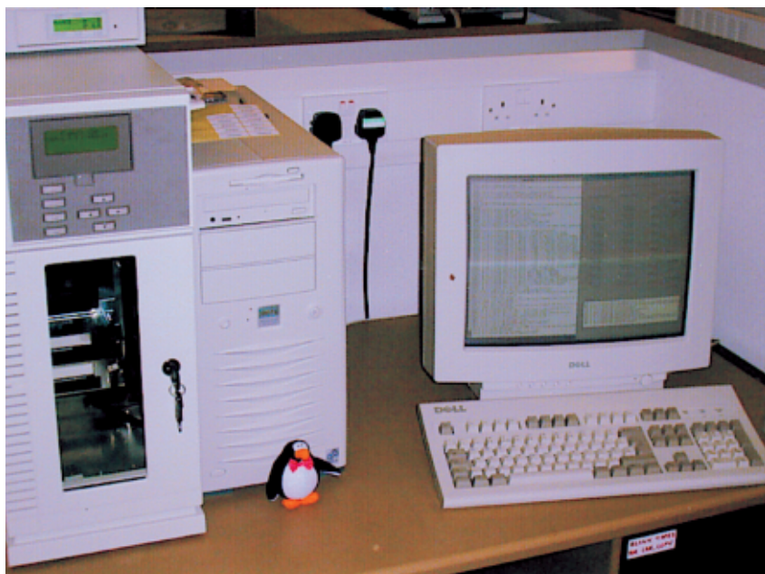
Figure 4. One of the UK-PAF data-processing sub-systems. The unit on the left is a robotic cassette-handling facility enabling continuous data processing
