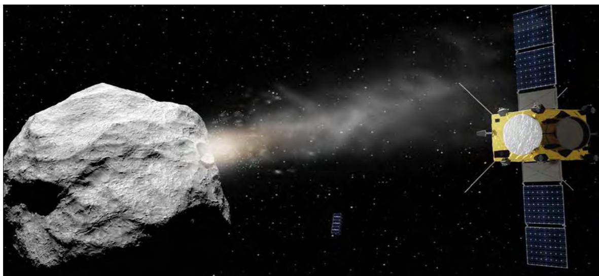
2 Illustration of the AIM spacecraft and deployed CubeSats at asteroid Didymos during the DART hypervelocity impact. (ESA)
