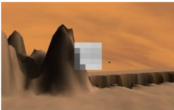
Figure 2. Example of the vision system of the robots, which consists in a 5x5 matrix of foveal cells whose receptive fields receive input from a gray level image of a limited area (100x100 pixels) of the whole image. The entire image is 640x480 pixels.
